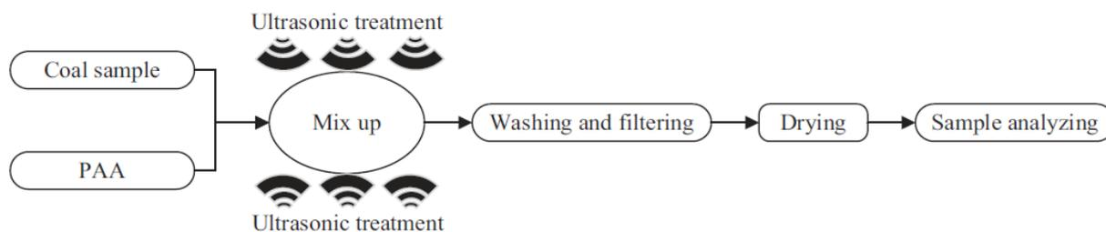
**Fig. 1.** The experimental procedure of coal desulfurization [16]
