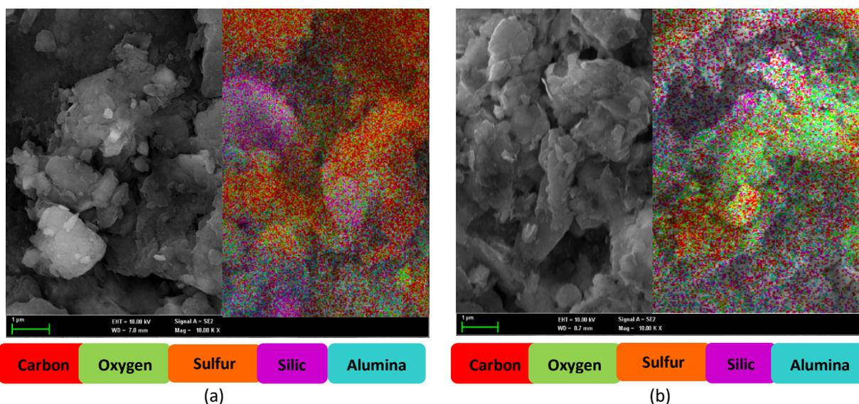
**Fig. 3.** SEM Image with mapping of elementary composition of (a) sulfur for raw coal and (b) treated coal at optimum condition for 30 minutes at 30°C
