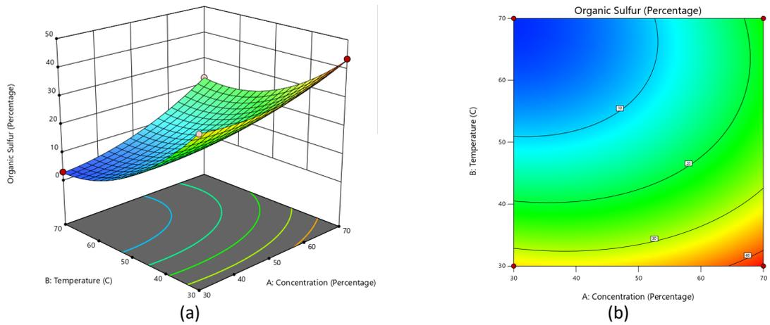
**Fig. 7.** Effect of concentration ratio and temperature on percentage sulfur removal (a) contour plot (b) surface plot
