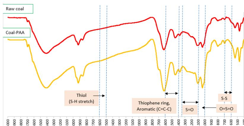
**Fig. 5.** FTIR results of raw coal and coal with PAA (70:30) at 30°C for 30 minutes
