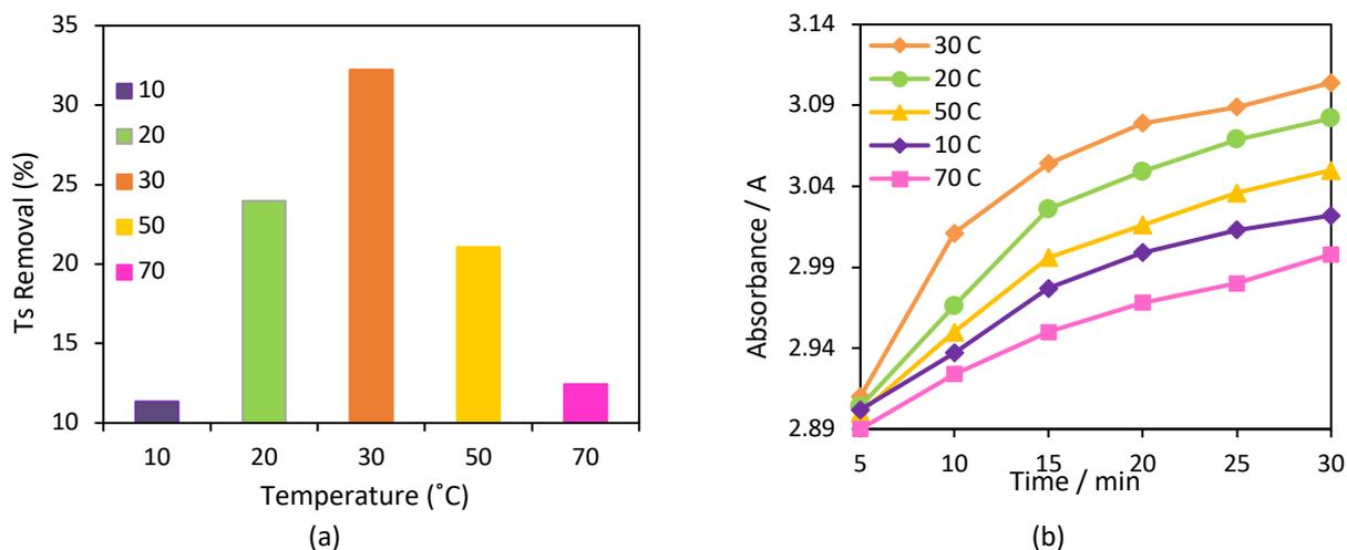
**Fig. 11.** Effect of ultrasonic temperature on the (a) total sulfur removal and (b) the production of  $\cdot\text{OH}$ , concentration ratio (70:30), sonication time (30 min)
