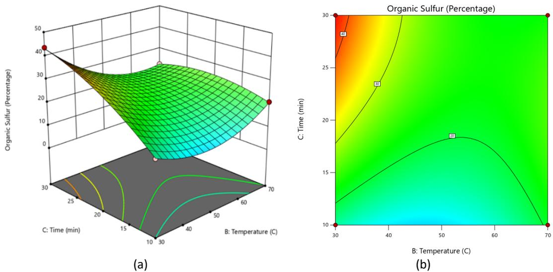
**Fig. 8.** Effect of temperature and time on percentage sulfur removal (a) contour plot (b) surface plot
