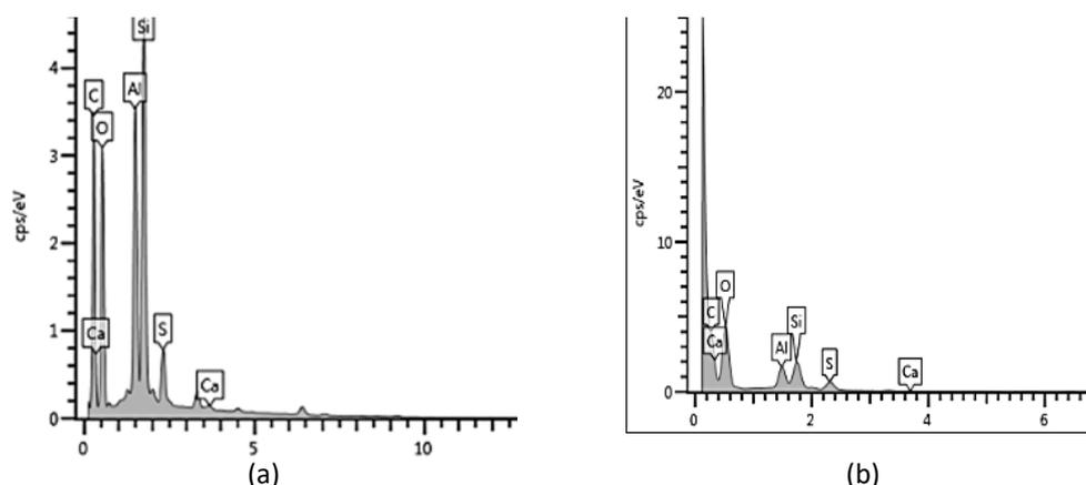
**Fig. 4.** EDX analysis of (a) raw coal and (b) treated coal at optimum condition at concentration ratio (70:30), for 30 minutes at 30°C
