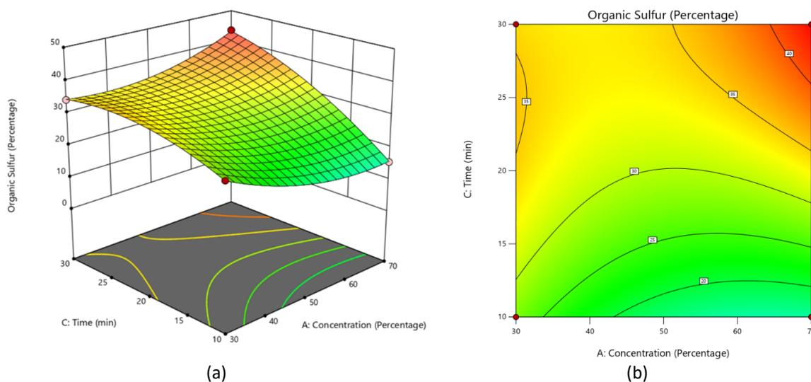
**Fig. 9.** Effect of concentration ratio and time on percentage sulfur removal (a) contour plot (b) surface plot
