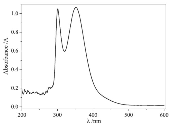
**Fig. 2.** The absorption spectra of KI solution after ultrasonic irradiation
