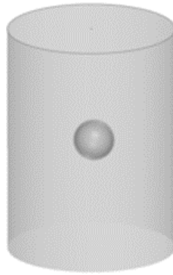
Fig. 3. Heat transfer fluid tank with PCM encapsulated sphere
