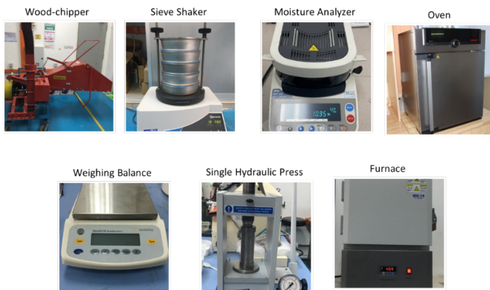
Fig. 1. Equipment involved in the khaya energy pellets production quality
