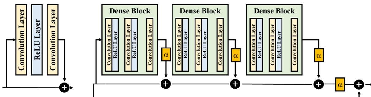
Fig. 1. Left: Residual block. Right: RRDB with upscaling
