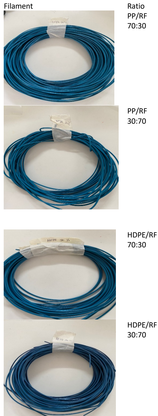
Fig. 1. 3D printer filament of HDPE/RF and PP/RF blends ratio
