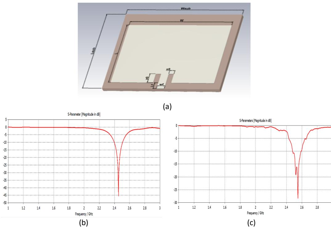
**Fig. 3.** (a) Single element MSPA, The return loss in dB (b) In free space (c) with breast tissue present
