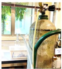
**Fig. 2.** Nitrogen bubbling process conducted following filtration
