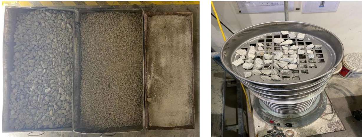
(a) coarse aggregate, fine aggregate, and mineral filler (b) Sieved aggregate according to 12.5 NMAS Fig. 1. Coarse aggregate, fine aggregate, and mineral filler content (b) Sieved aggregate according to 12.5 NMAS
