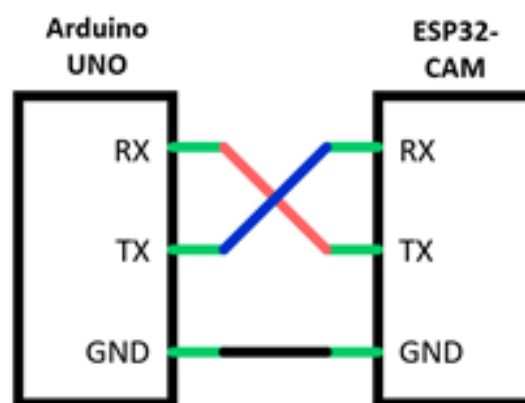
Fig. 8. Universal Asynchronous Receive Transmit (UART) communication between Arduino UNO and ESP32-CAM
