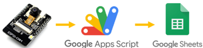
Fig. 9. Using Google Apps Script to publish readings on Google Sheets
