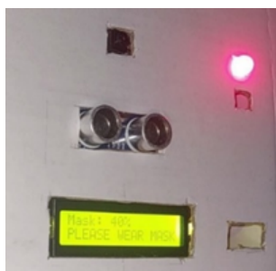
Fig. 20. LCD and red LED being lit when mask is not properly worn
