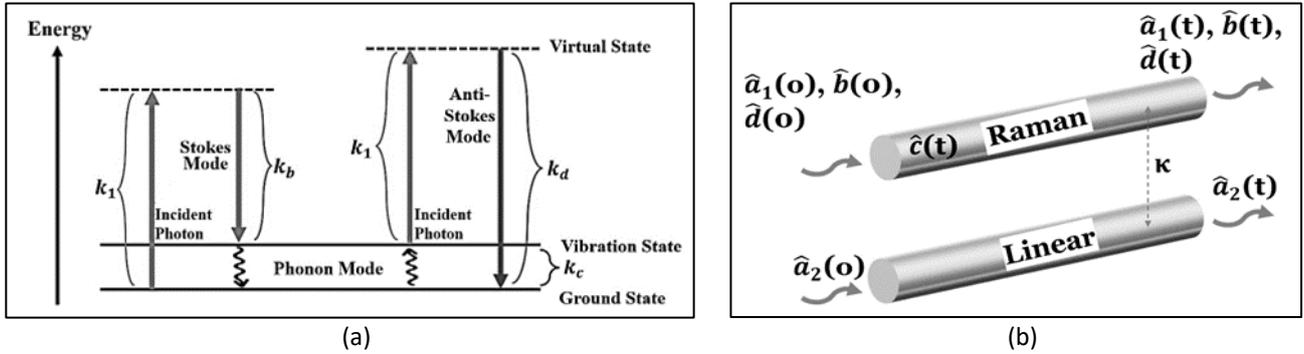
Fig. 1. (a) Diagram for Raman process (b) Basic diagram of the two-waveguide asymmetric nonlinear coupler
