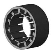
**Fig. 1.** SMC Stator elaborated by Muthusamy *et al.,* [14]
