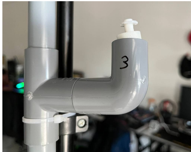
Fig. 7. Float sensor attachment method
