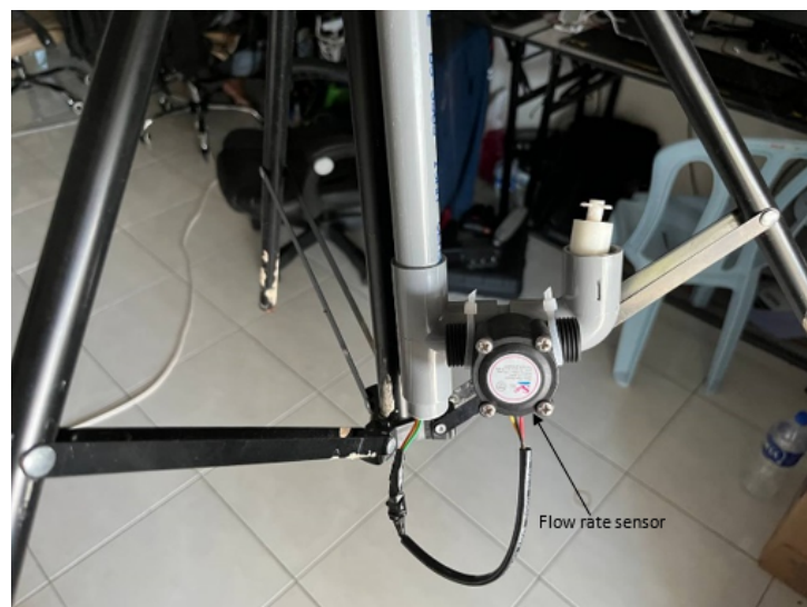
Fig. 9. Flow Rate Sensor Attachment Method
