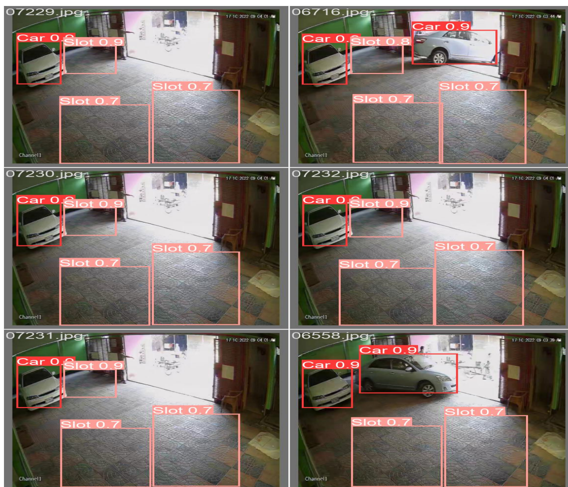
Fig. 7. The image shows the performance of YOLOv5 when used to identify cars and slots
