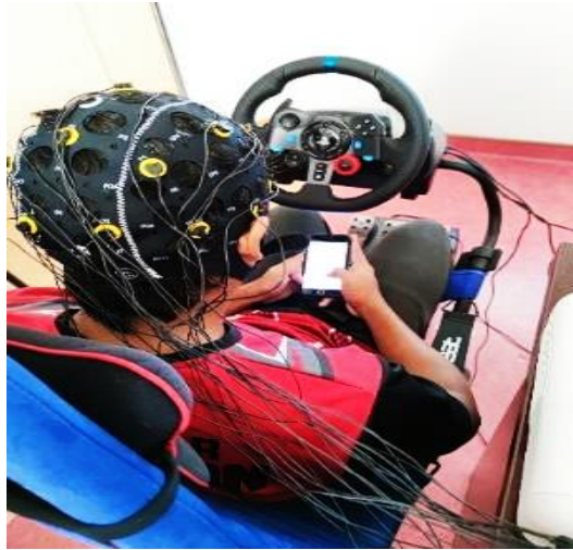
Fig. 2. A participant is wearing a 19-channels DABO EEG electrode cap
