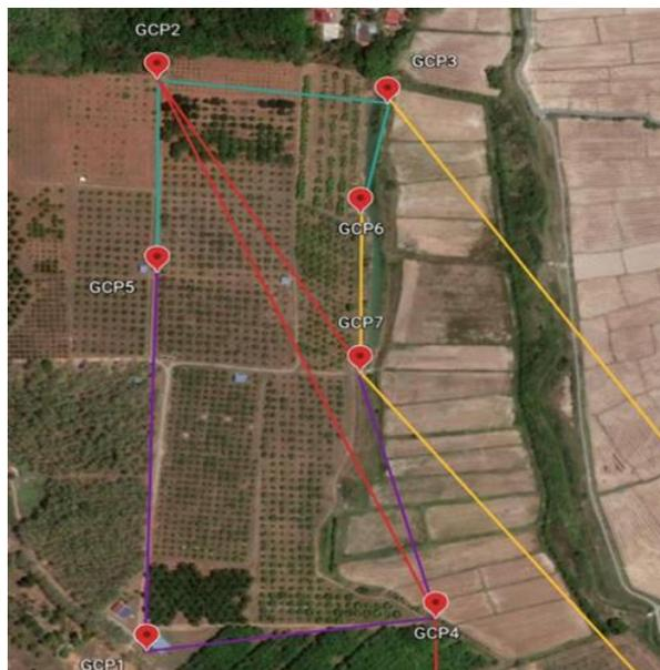
Fig. 4. Network design of GCPs
