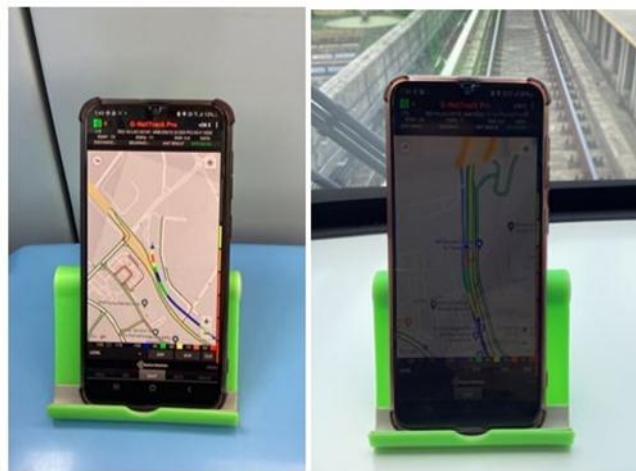
Fig. 5. Set up of UE during drive test
