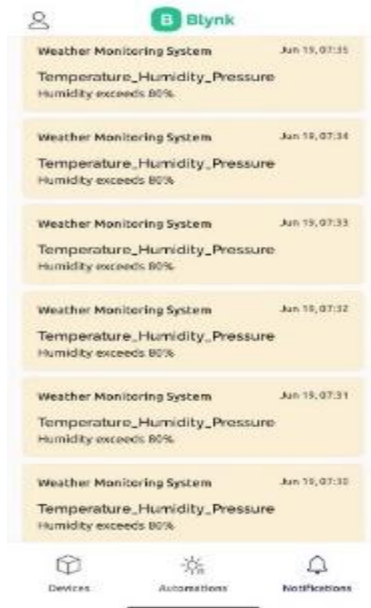
Fig. 8. Example of alarm notification on Blynk when meteorological parameters above/below the thresholds set.
