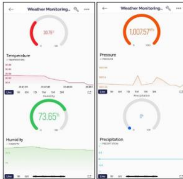
Fig. 4. Weather monitoring system IoT dashboard
