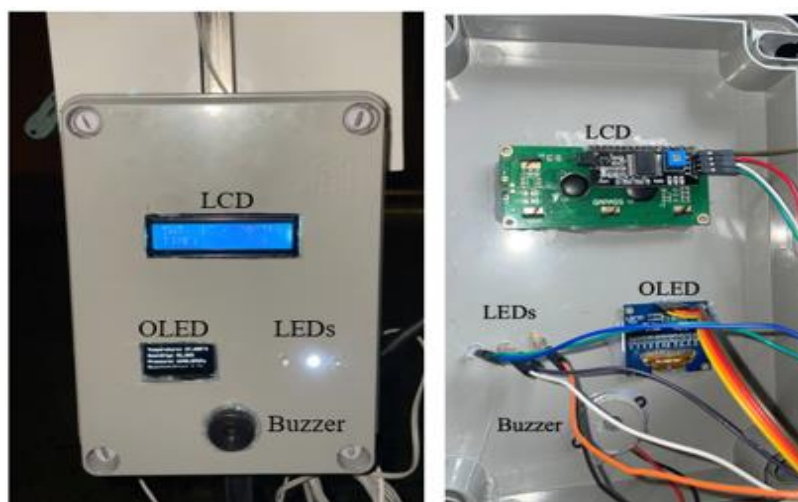
Fig. 9. Alarm & notification features on the proposed weather monitoring system
