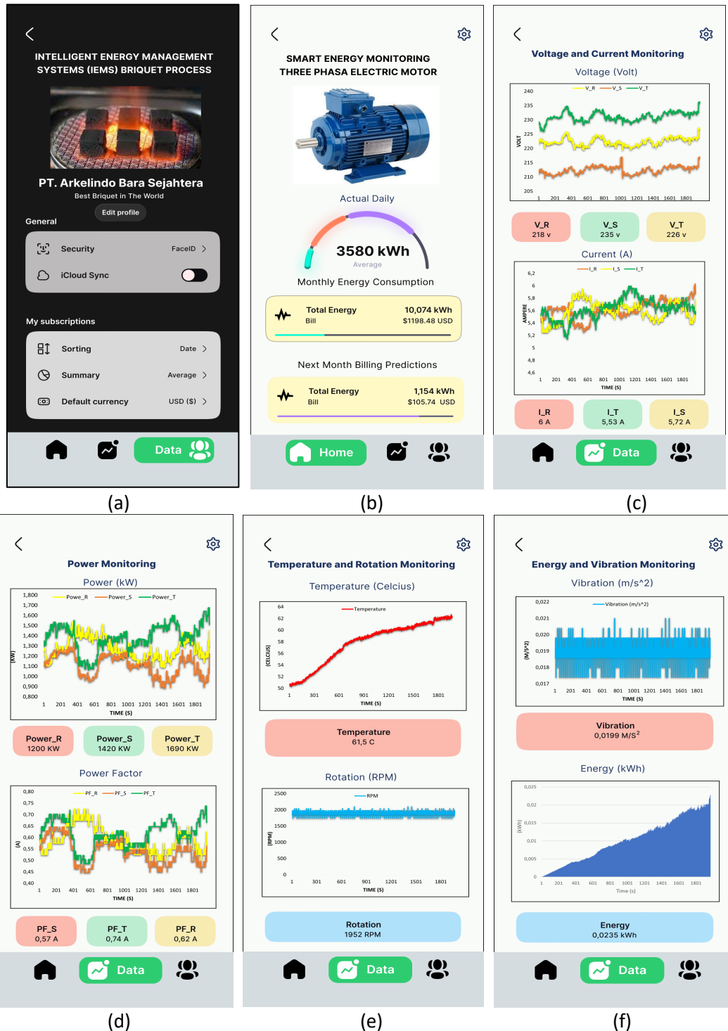
Fig. 11. IoT platform of energy monitoring for three phase induction motor: (a) home section, (b) real time monitoring, (c) voltage and current monitoring, (d) power monitoring, (e) temperature and rotation monitoring, (f) energy and vibration monitoring
