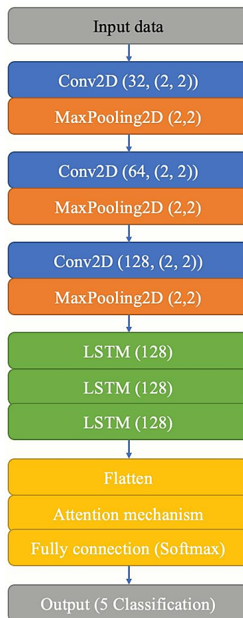
Fig. 5. The structure of the proposed CNN-LSTM-SA
