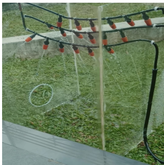
Fig. 7. Sprayer multi-level (three level) system
