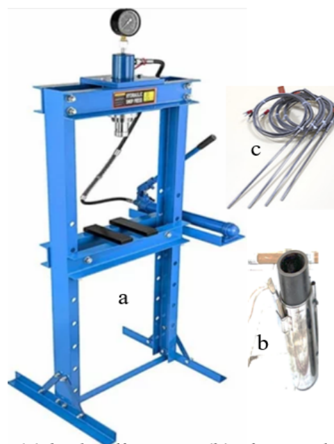
(a) hydraulic press, (b) pipes and heaters, (c) thermocouple
