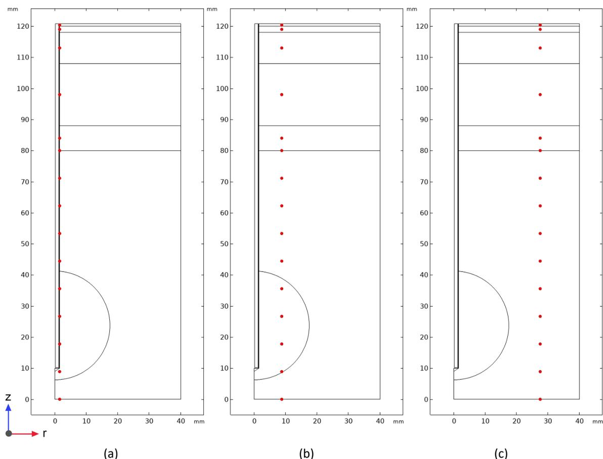
Fig. 2. Temperature probe placement for data extraction at (a)  $r = 1.51$ , (b)  $r = 8.75$ , (c)  $r = 27.5$
