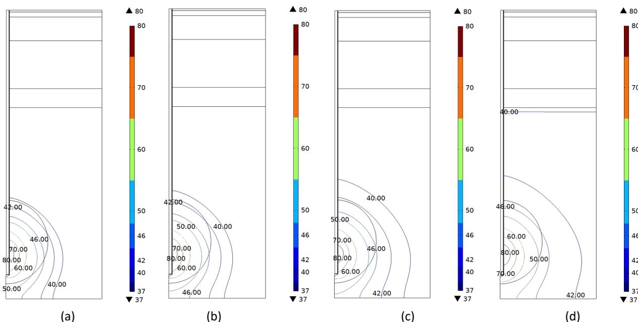
**Fig. 6.** Temperature distribution contour on  $t = 10$  min with variations; (a)  $Q_m = 368,1 \text{ W/m}^3$ ; (b)  $Q_m = 7000 \text{ W/m}^3$ ; (c)  $Q_m = 14000 \text{ W/m}^3$ ; (d)  $Q_m = 29000 \text{ W/m}^3$
