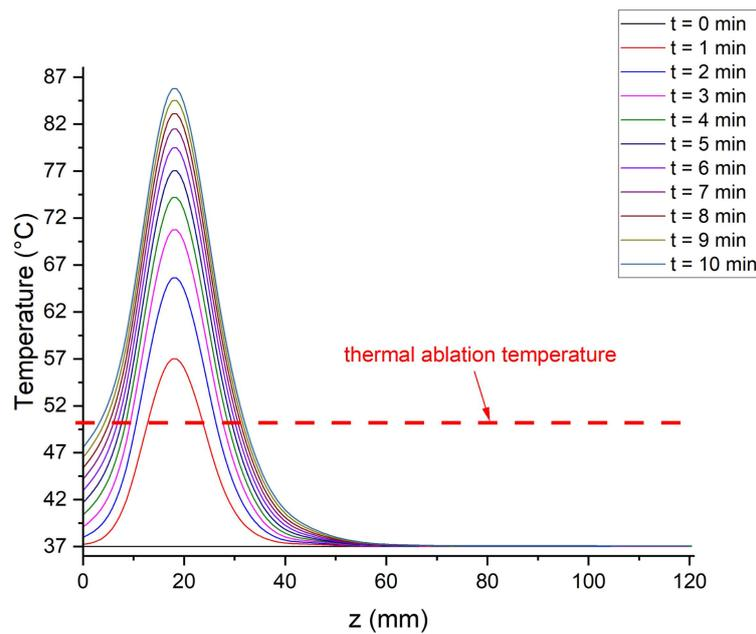
**Fig. 3.** Temperature distribution on microwave ablation therapy along  $r = 1,51$  and  $Q_m = 368,1 \text{ W/m}^3$
