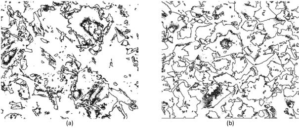
Fig.5. Pore map (a) BAC (b) BAC+NaOH
