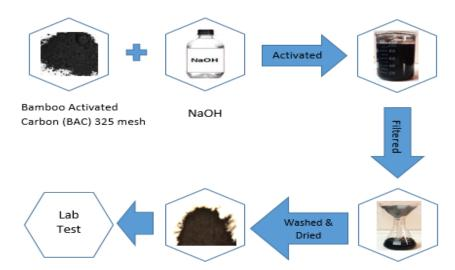
Fig. 2. Bamboo-activated carbon activation material preparation procedure
