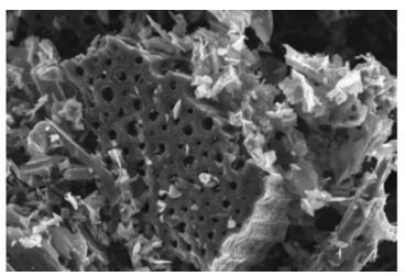
Fig. 1. The pore structure of bamboo activated carbon [17]
