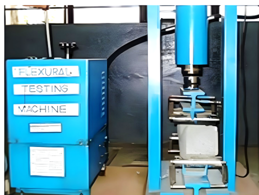
Fig. 8. Flexural strength testing of sample
