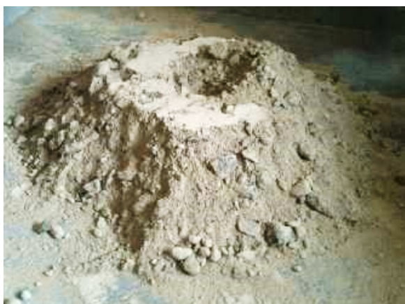
Fig. 5. Proportions of concrete materials with previously added solution
