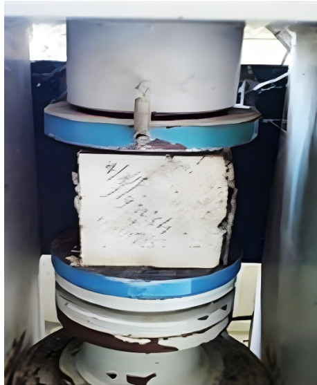
Fig. 9. Testing of split tensile strength
