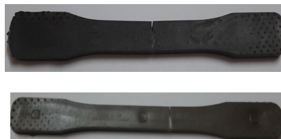
Fig. 2. Specimen ASTM D638
