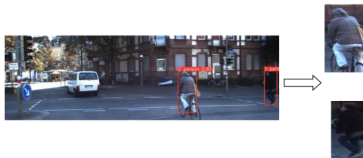
Fig. 2. Cropping the moving objects from each frame
