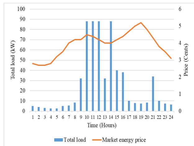
Fig. 3. Dynamic variation of market energy price and load demand throughout the day [22]
