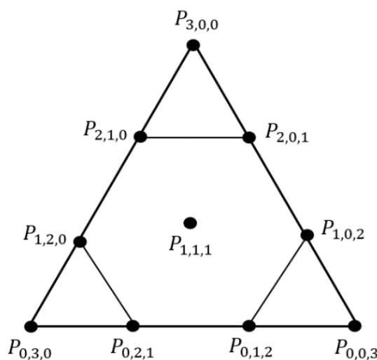
Fig. 4. Corner points for each tangent plane
