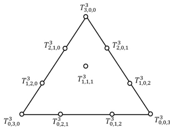
Fig. 3. Control Points over Triangular Domain
