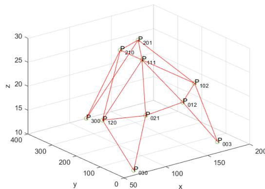
**Fig. 5.** Control Polygon in 3D Space
