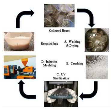
Fig. 1. Stages of the recycling process
