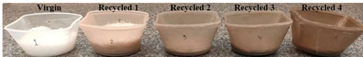
Fig. 5. Samples from virgin PP and four recycling cycles
