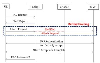
Fig. 4. MitM Control deplete assault devices
