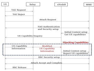
Fig. 3. MITM capability hijacking attack
