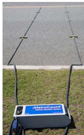
Fig. 1. Temporary sensor installed on a road
