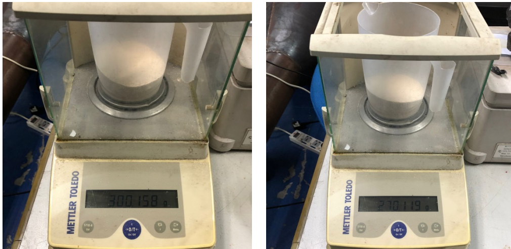
Fig. 3. Weight of particle injected (left) and particle collected on collection tank (right) for the testing and commissioning experiment
