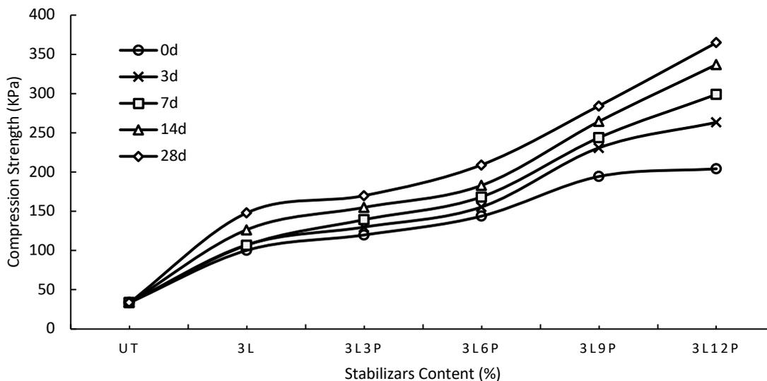
Fig. 2. Strength of treated soil with different SH-85 content[24]
