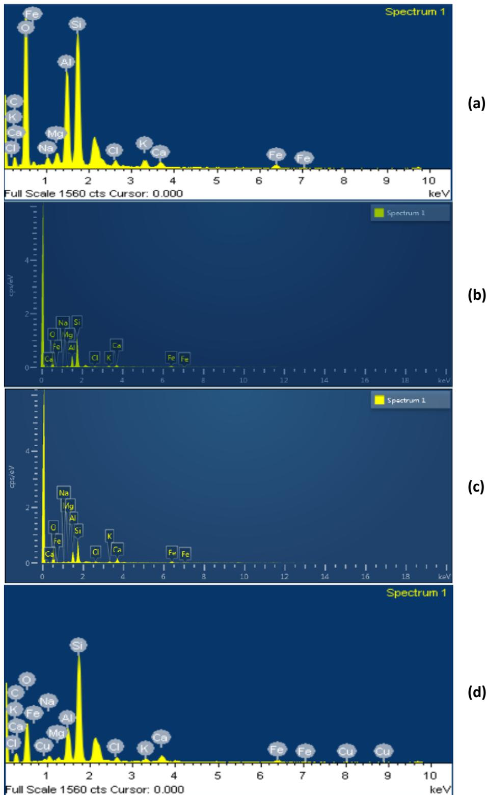
**Fig. 5.** EDAX spectrums of untreated (a) and 3L9P at different curing intervals, 7 days (b), 14 days (c) and 28 days (d)
