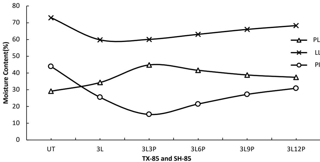
Fig. 1. Atterberg Limits of Batu Pahat Soft Clay soils after addition of Probase Stabilizers [24]
