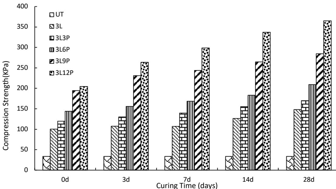
Fig. 3. Strength of treated soil with Probase Stabilizers content at different curing time[24]
