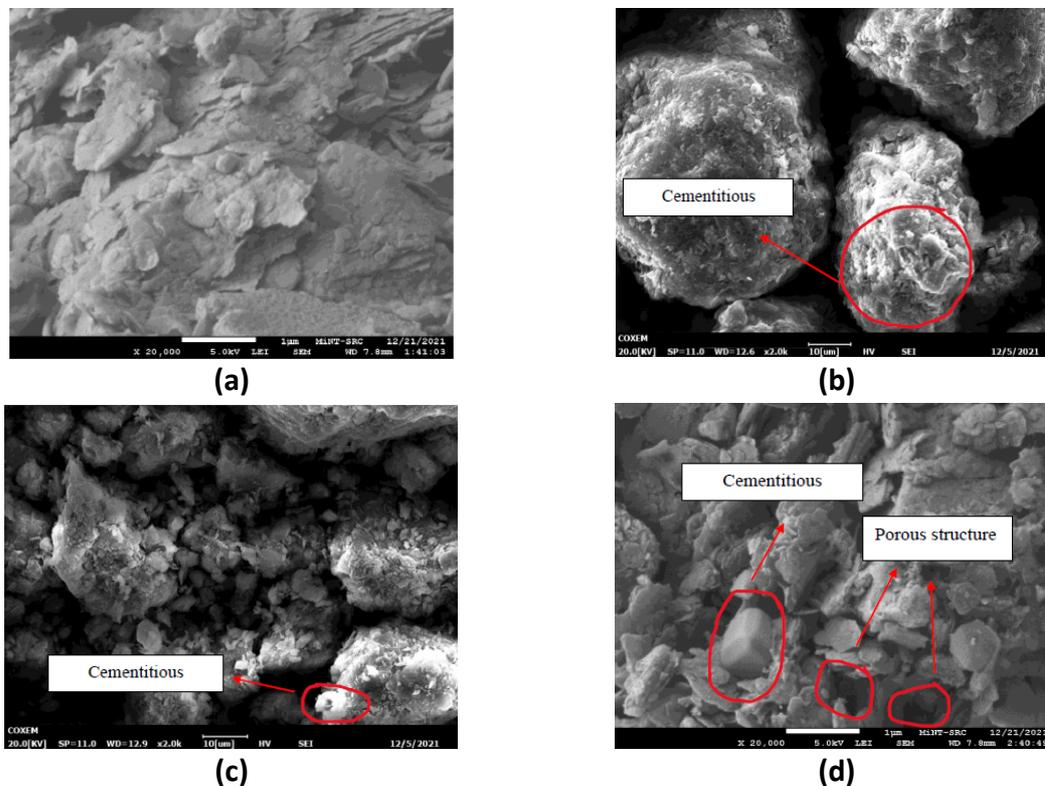
**Fig. 4.** Micrograph of untreated sample (a) and 3L9P at different curing intervals, 7 days (b), 14 days (c), and 28 days (d)
