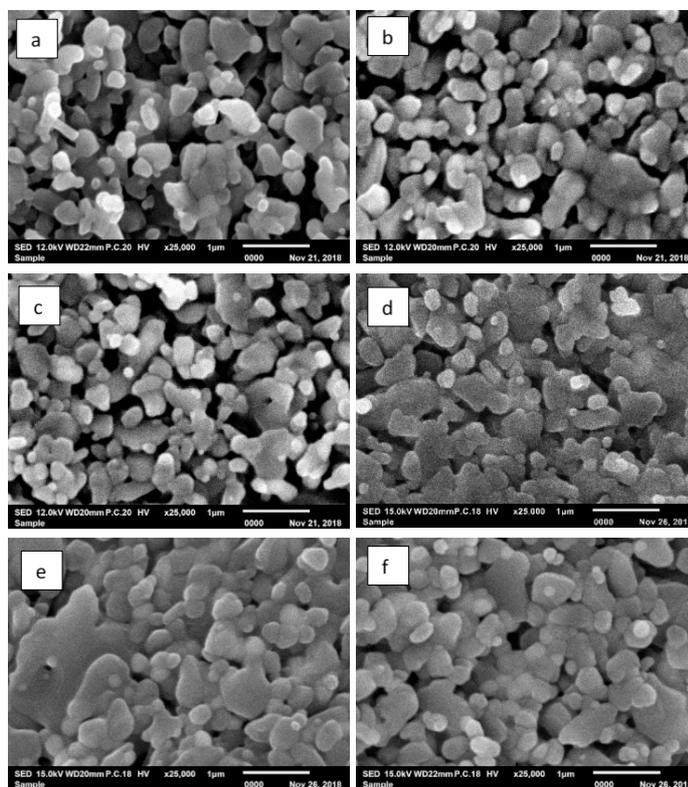
**Fig. 5.** Microstructure of ZTA-pyrolytic carbon ceramics composite subjected to different holding time of CVI at 25000 magnification (a) 0h, (b) 1h, (c) 1.5h, (d) 2h, (e) 2.5h, (f) 3h
