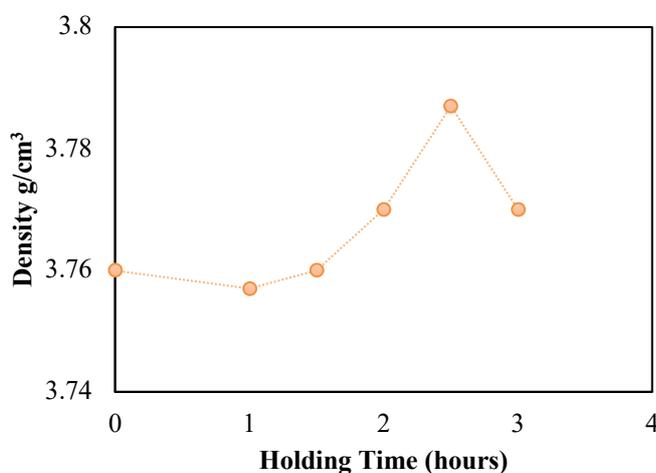
Fig. 6. Density of pyrolytic carbon infiltrated ZTA at different holding time
