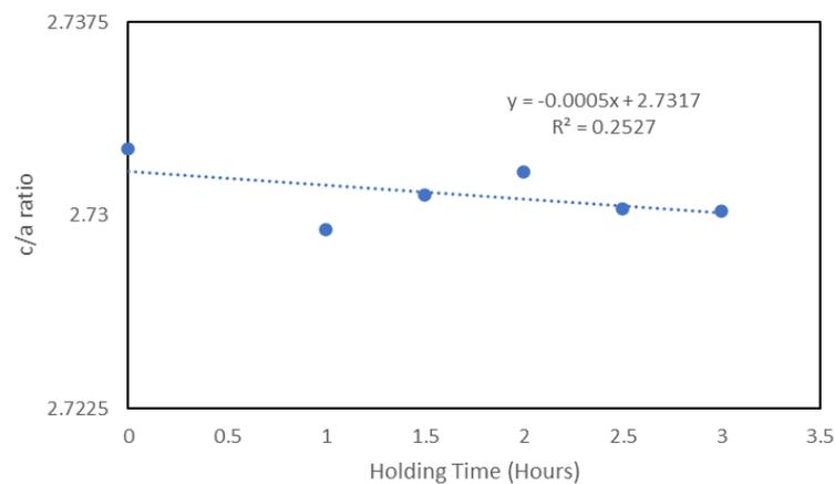
**Fig. 3.**  $c/a$  ratio as function at different holding time of CVI
