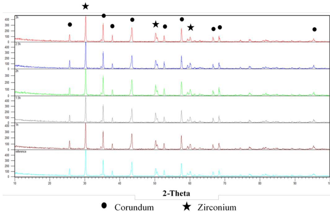
**Fig. 2.** X-ray diffraction analyses for ZTA-C samples with different holding time of CVI method
