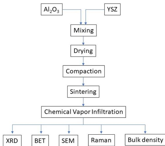
**Fig. 1.** Flowchart of the sample preparation and respective characterizations.
