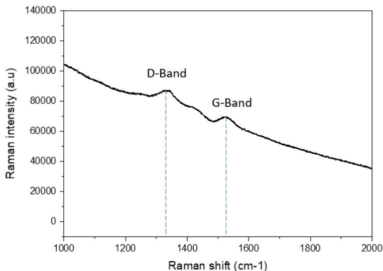
**Fig. 4.** Raman spectra of pyrolytic carbon in ZTA at 2 hours of holding time of CVI
