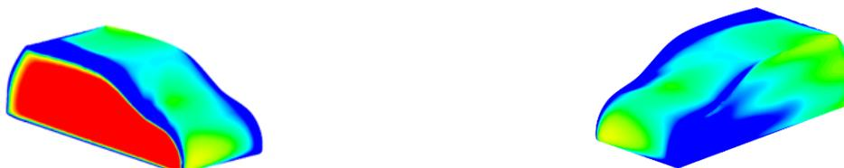
**Fig. 6.** The surface pressure contour of the compact car with various crosswind angles
