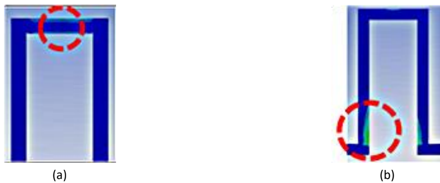
Fig. 9. Simulation of equivalent plastic strain (mm/mm) for rectangular pattern subjected to (a) longitudinal ( \epsilon_p = 0.063310 ) (b) lateral loading ( \epsilon_p = 0.013366 )
