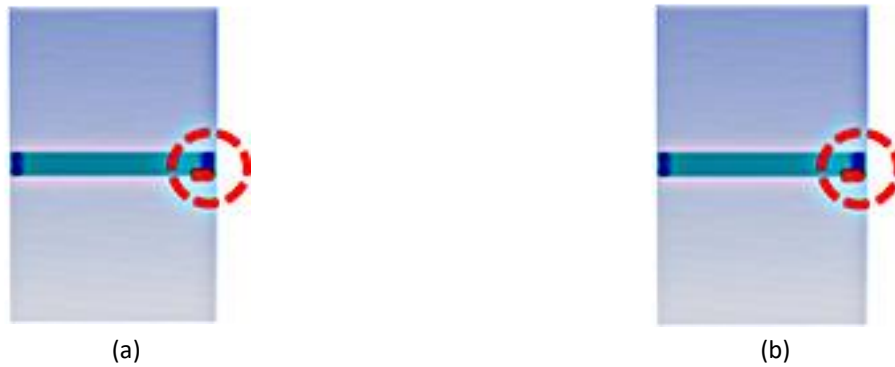
Fig. 8. Simulation of equivalent plastic strain (mm/mm) for straight pattern subjected to (a) longitudinal ( \epsilon_p = 0.311840 ) (b) lateral loading ( \epsilon_p = 0.000000 )
