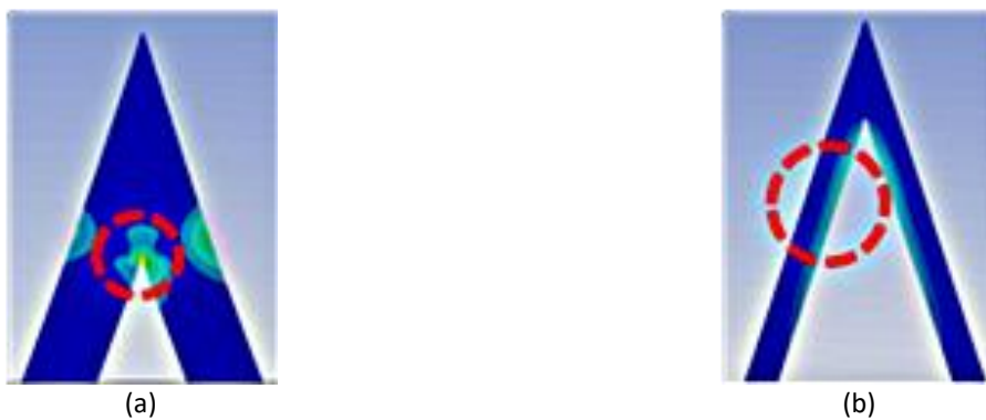
Fig. 4. Simulation of equivalent plastic strain (mm/mm) for zigzag pattern subjected to (a) longitudinal ( \epsilon_p = 0.056022 ) (b) lateral loading ( \epsilon_p = 0.013981 )
