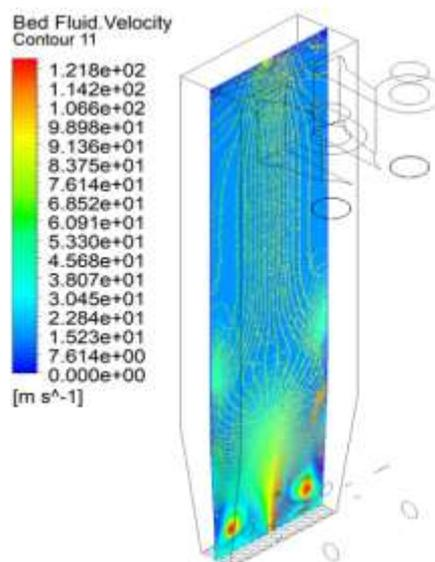
**Fig. 18.** Velocity profile based on velocity magnitude contours
