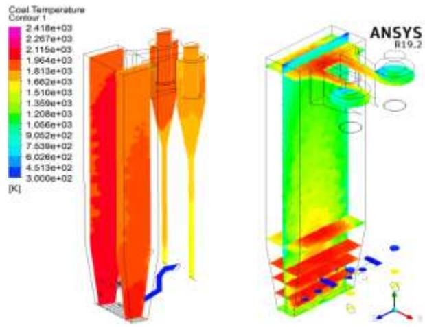
**Fig. 11.** Combustion temperature contour percentage of PKS mix 40%
