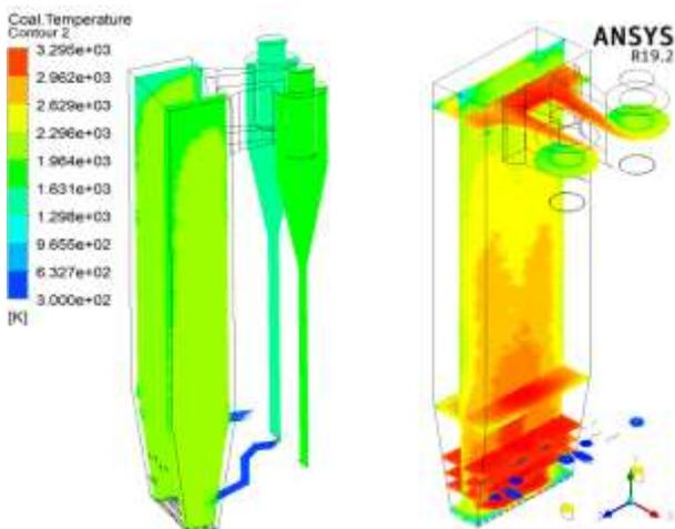
**Fig. 10.** Combustion temperature contour percentage of PKS mix 20%
