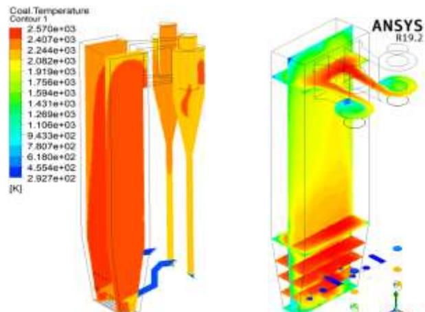
**Fig. 13.** Combustion temperature contour percentage of PKS mix 80%
