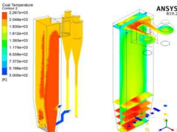
**Fig. 12.** Combustion temperature contour percentage of PKS mix 60%
