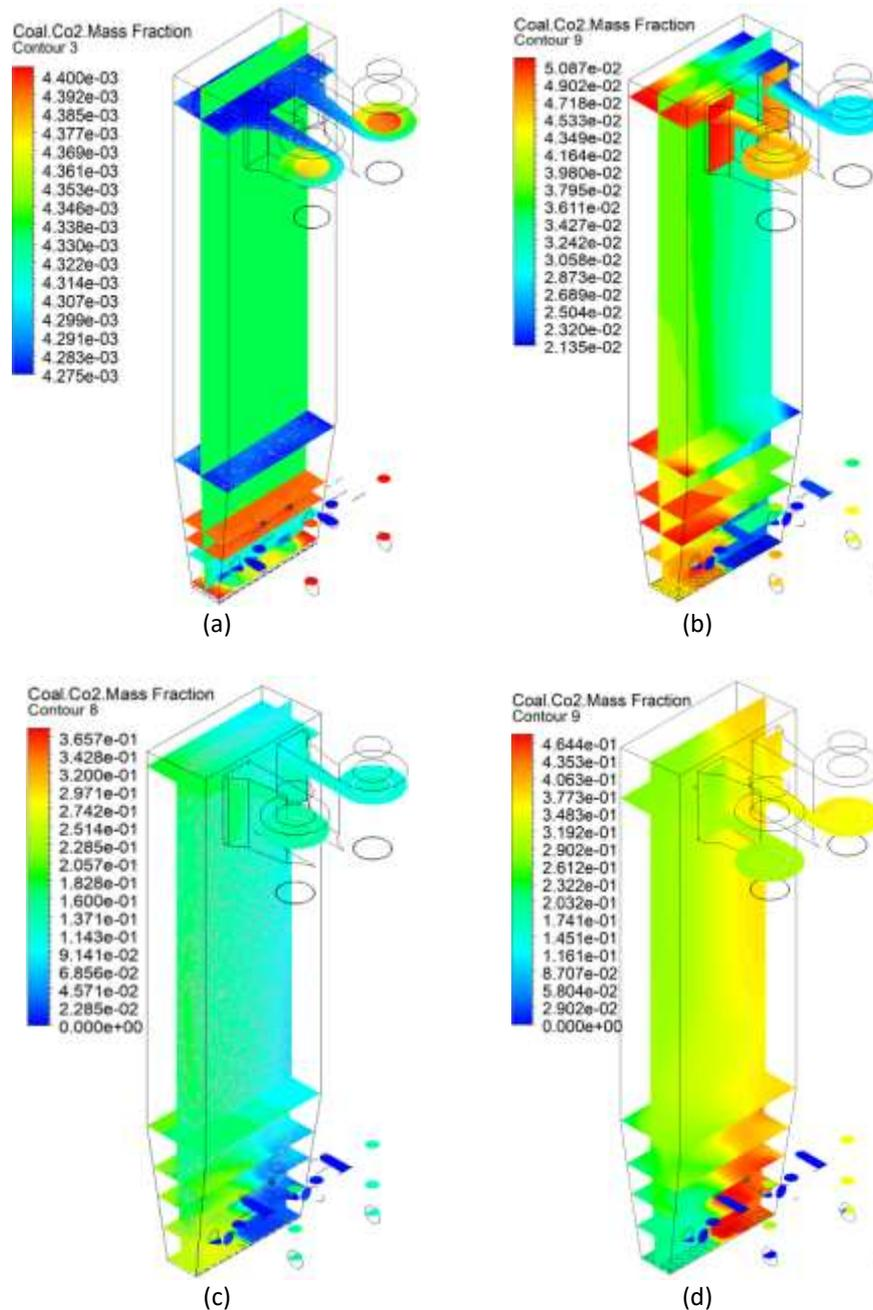
**Fig. 16.** CO<sub>2</sub> mass fraction contour (a) variation 20% (b) variation 40% (c) variation 60% (d) variation 80%
