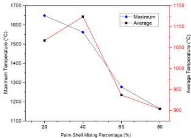
**Fig. 14.** Maximum and average temperature at Furnace Bed Temperature (FBT)
