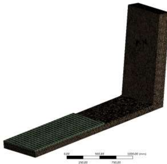
Fig. 2. Wire mesh geometry of solar chimney-collector with fins for solar PV cooling
