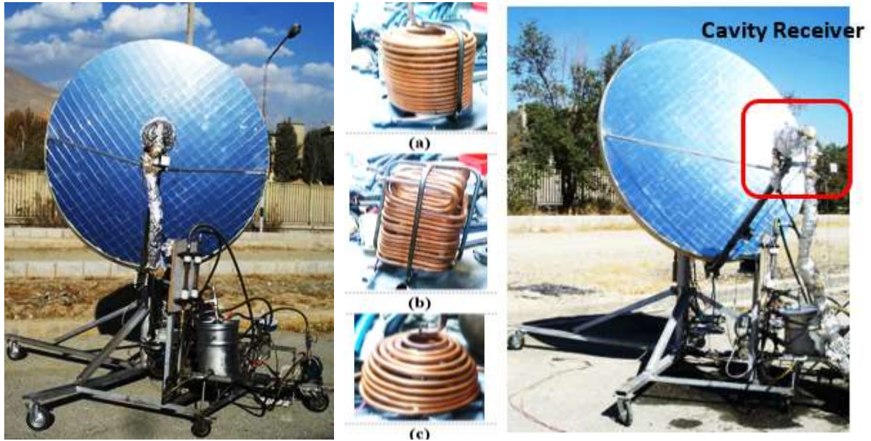
Fig. 1. A view of the solar dish concentrator and the wounded cavity receivers with copper tube including a) cylindrical, b) cubical, and c) hemispherical cavity receiver
