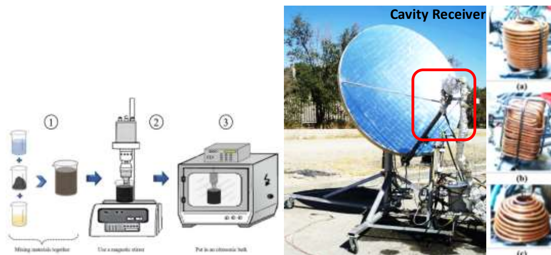
Fig. 1. (left) Process of the Al 2 O 3 nanoparticles preparation, (right) A view of the solar dish concentrator and the wounded cavity receivers with copper tube including a) cylindrical, b) cubical, and c) hemispherical cavity receiver
