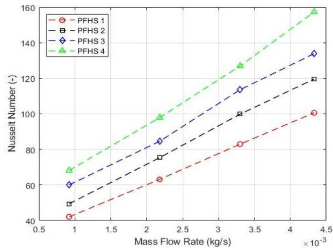
**Fig. 8.** Nusselt Number for different designs subjected to parallel flow at different flow rates
