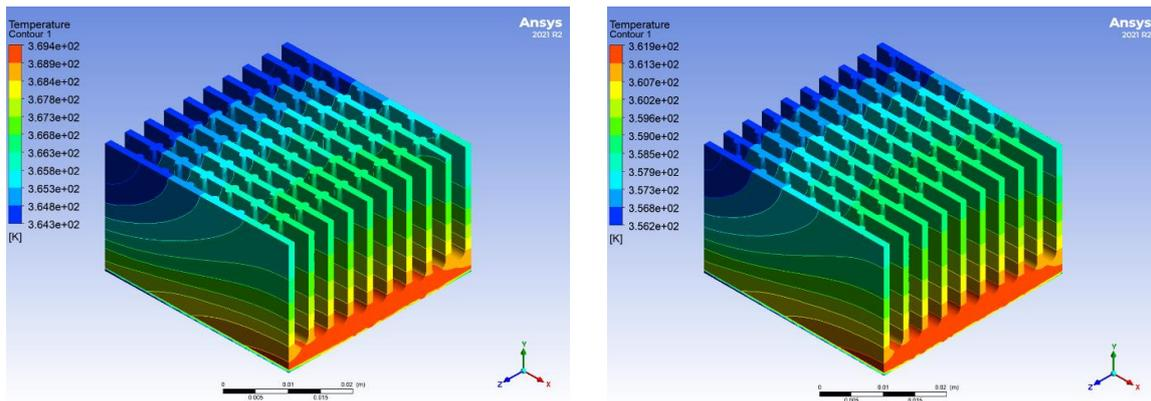
(c) Plate-fin heat sinks with fillet profile and symmetrical half-round pins (PFHS 3) (d) Plate-fin heat sinks with fillet profile and corrugated half-round pins (PFHS 4)
