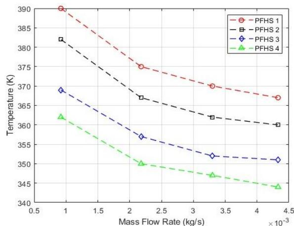
**Fig. 6.** The base temperature for different designs subjected to parallel flow at different flow rates
