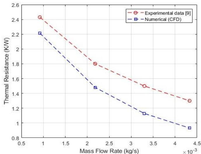
**Fig. 4.** Validation of numerical approach (CFD) at different mass flow rates for thermal resistance
