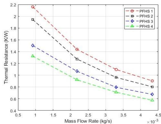
**Fig. 7.** The thermal resistance for different designs subjected to parallel flow at different flow rates
