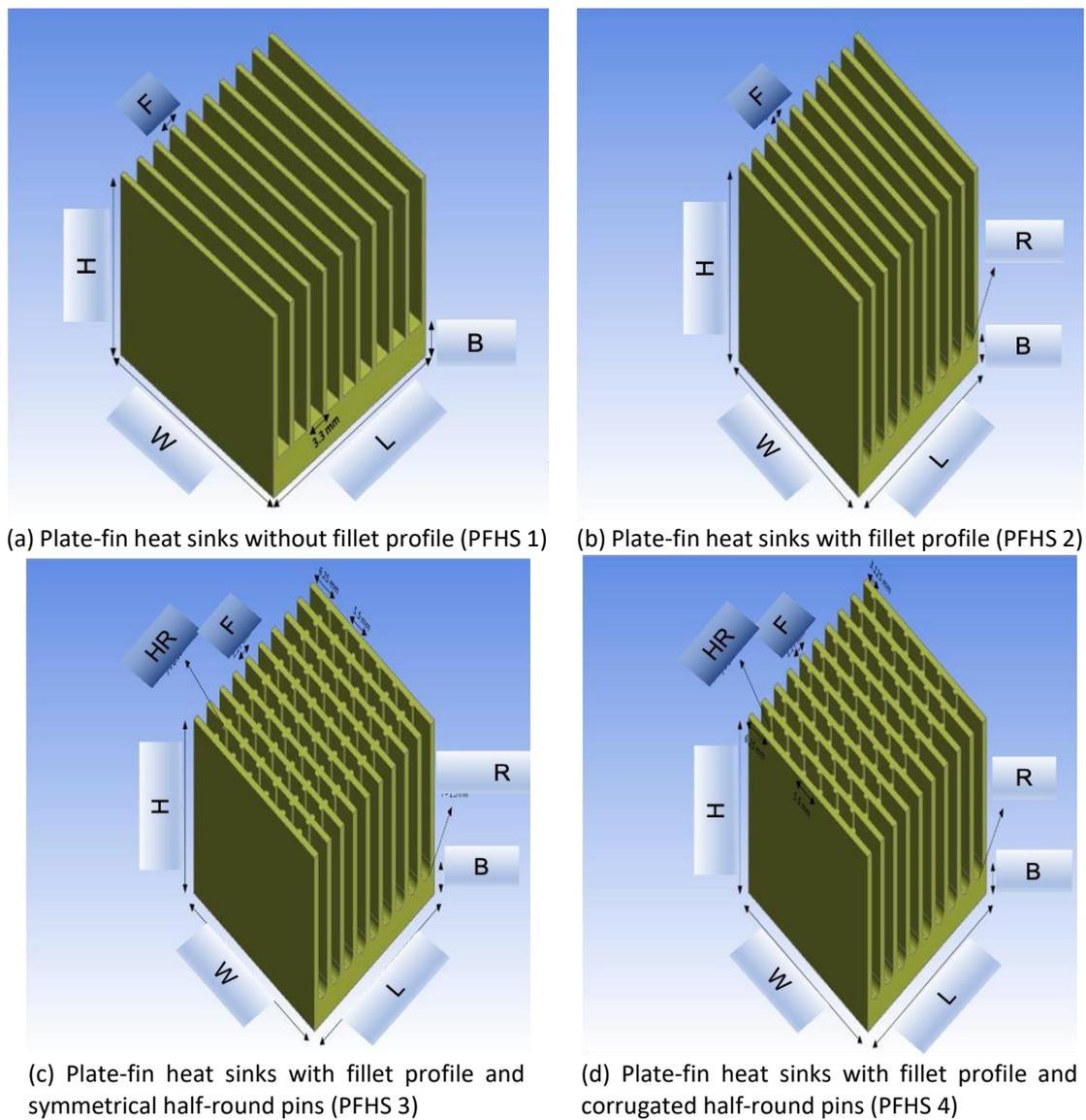
**Fig. 1.** Geometrical model of plate-fin heat sinks
