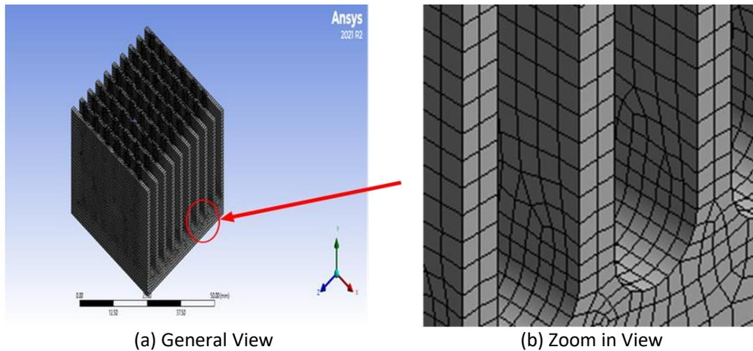
**Fig. 2.** Meshing configuration
