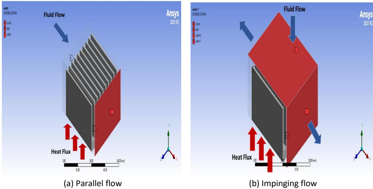
Fig. 3. Numerical analysis of computational domain with boundary conditions
