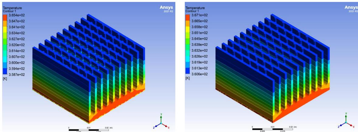
(c) Plate-fin heat sinks with fillet profile and symmetrical half-round pins (PFHS 3) (d) Plate-fin heat sinks with fillet profile and corrugated half-round pins (PFHS 4)
