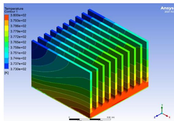
(b) Plate-fin heat sinks with fillet profile (PFHS 2)
