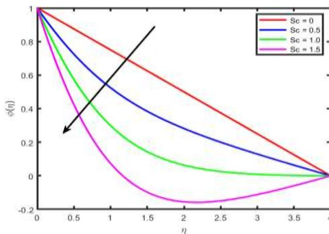
**Fig. 12.** Effect of  $S_c$  Schmidt number on  $\phi(\eta)$
