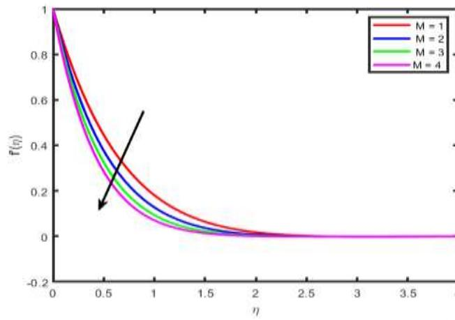
Fig. 1. Effect of M (weak magnetic strength) on  $f'(\eta)$
