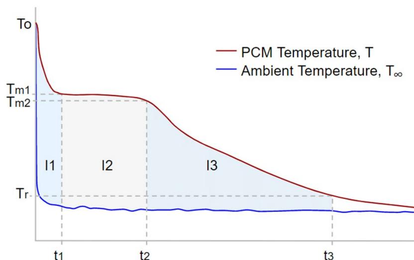
**Fig. 2.** Variation of fluid temperature with time for different phase change materials
