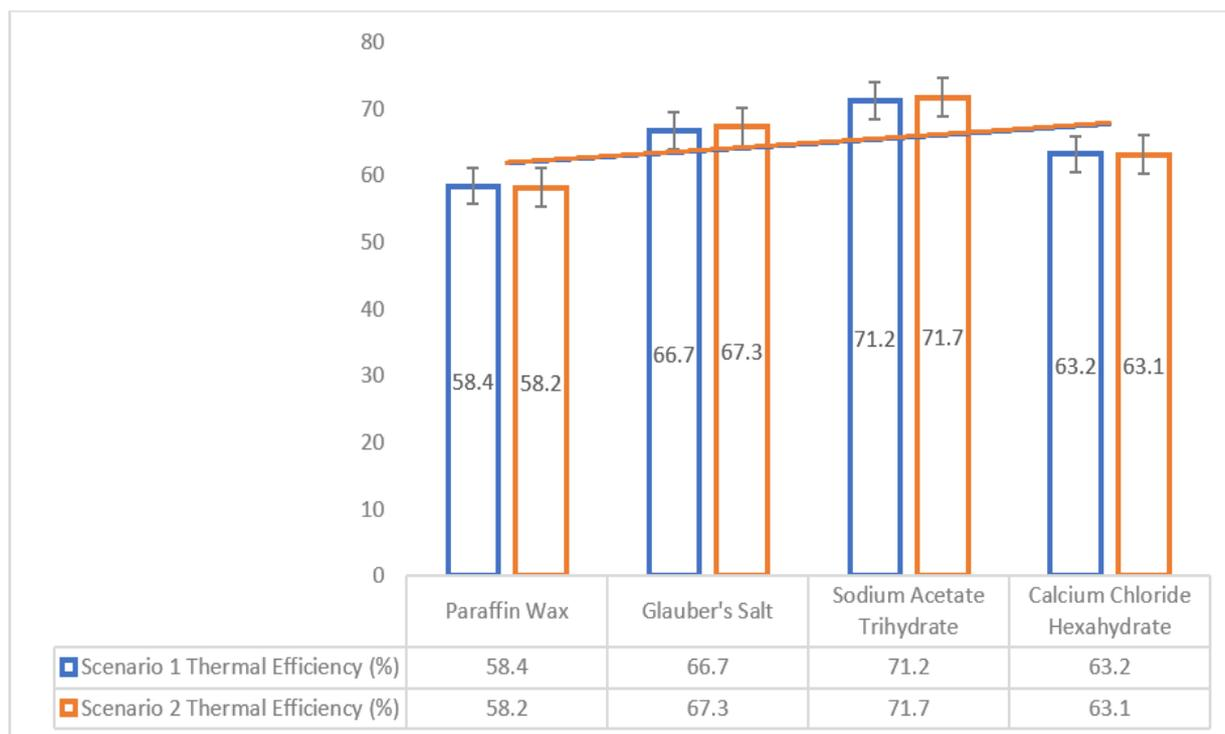
**Fig. 3.** Impact of phase change material placement on collector performance
