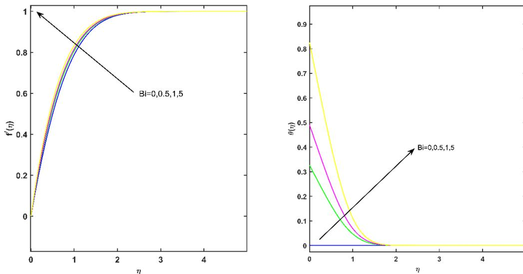
Fig. 5. Velocity profile  $f'(\eta)$  and temperature profile  $\theta(\eta)$  for various value of  $Bi$
