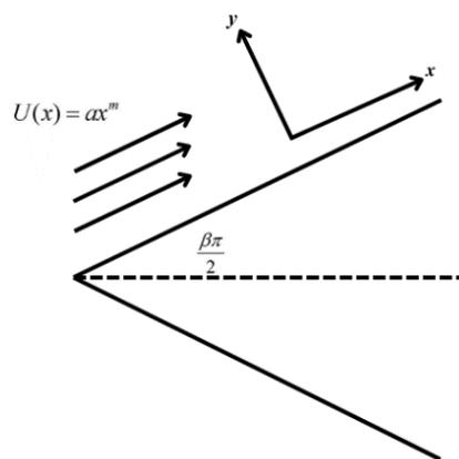
**Fig. 1.** Schematic diagram of mixed convection flow of nanofluid over a static wedge
