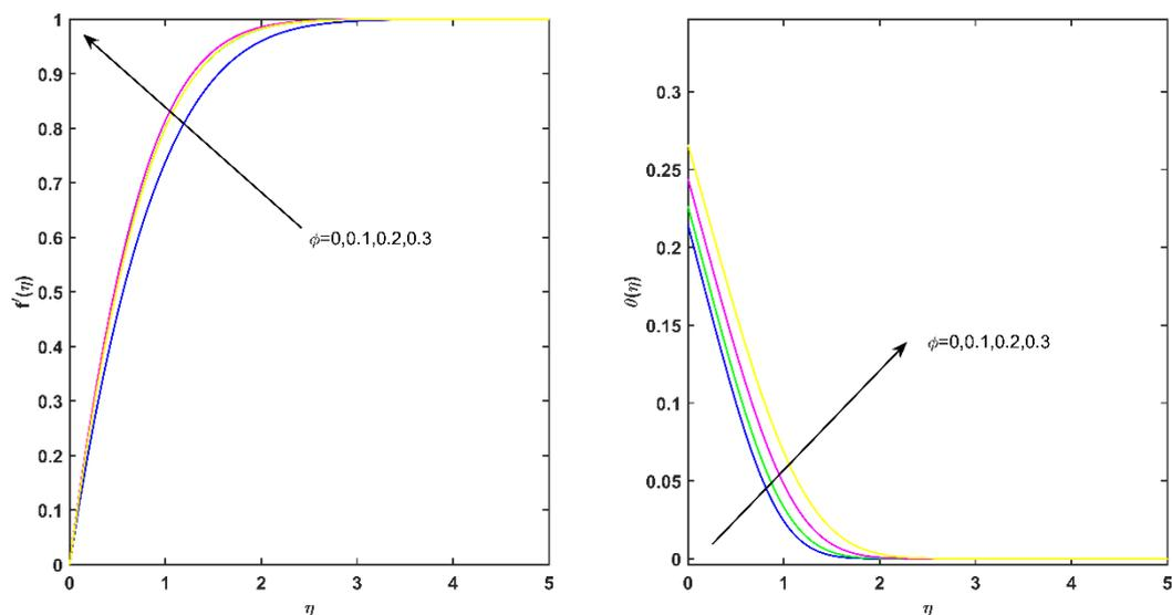
**Fig. 4.** Velocity profile  $f'(\eta)$  and temperature profile  $\theta(\eta)$  for various value of  $\phi$
