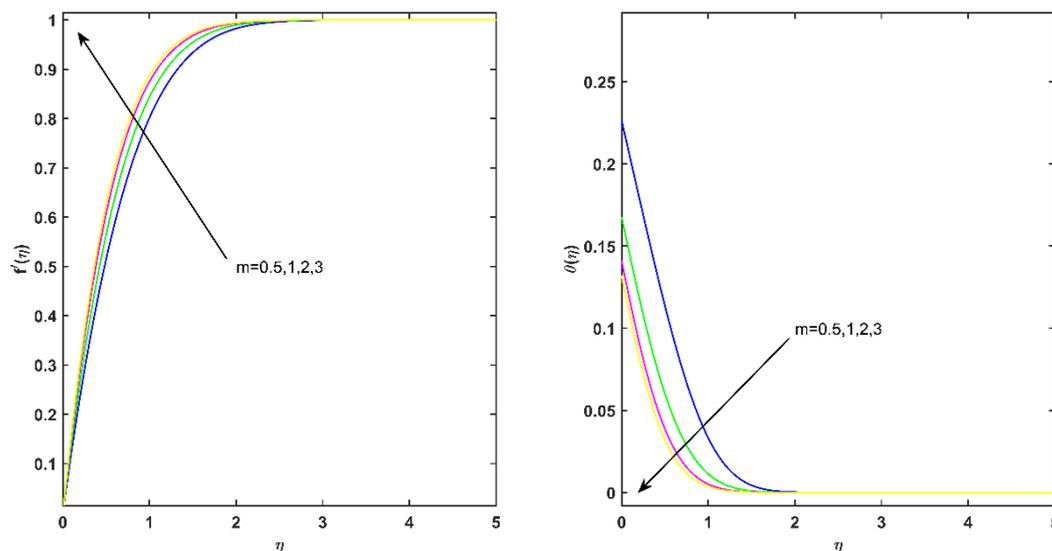
**Fig. 2.** Velocity profile  $f'(\eta)$  and temperature profile  $\theta(\eta)$  for various value of  $m$
