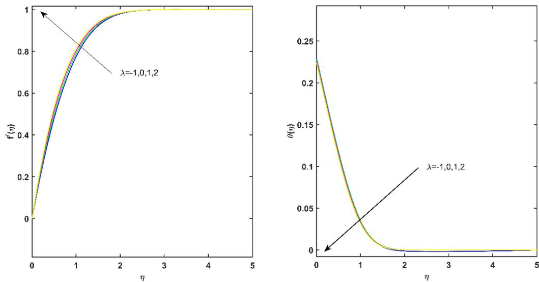
**Fig. 3.** Velocity profile  $f'(\eta)$  and temperature profile  $\theta(\eta)$  for various value of  $\lambda$
