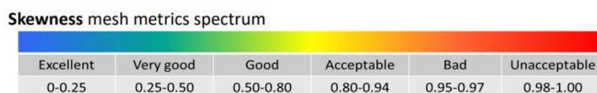
Fig. 7. Skewness mesh metrics spectrum [17]
