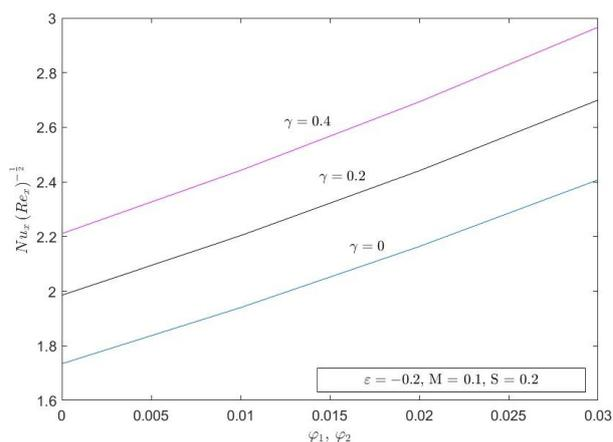
**Fig. 13.** Effect of curvature parameter,  $\gamma$  on local Nusselt number  $Nu_x(Re_x)^{-\frac{1}{2}}$
