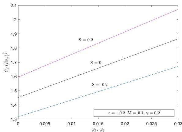
**Fig. 14.** Effect of suction,  $S$  on local skin friction  $C_f(Re_x)^{\frac{1}{2}}$
