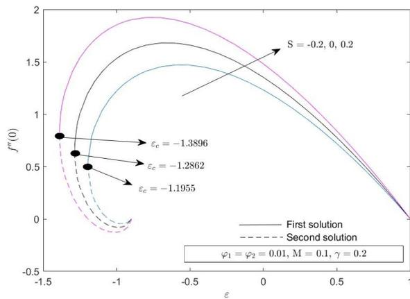
**Fig. 8.** Effect of suction,  $S$  on reduced skin friction  $f''(0)$
