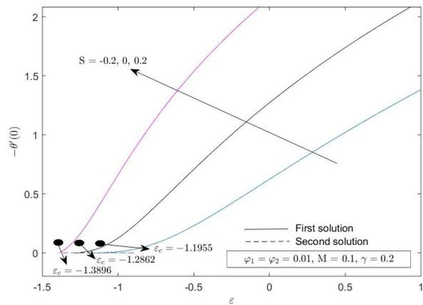
**Fig. 9.** Effect of suction,  $S$  on reduced heat transfer  $-\theta'(0)$
