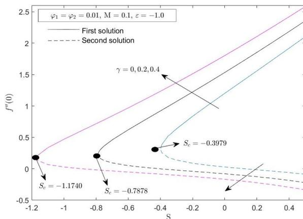
**Fig. 10.** Effect of curvature parameter,  $\gamma$  with suction,  $S$  on reduced skin friction  $f''(0)$
