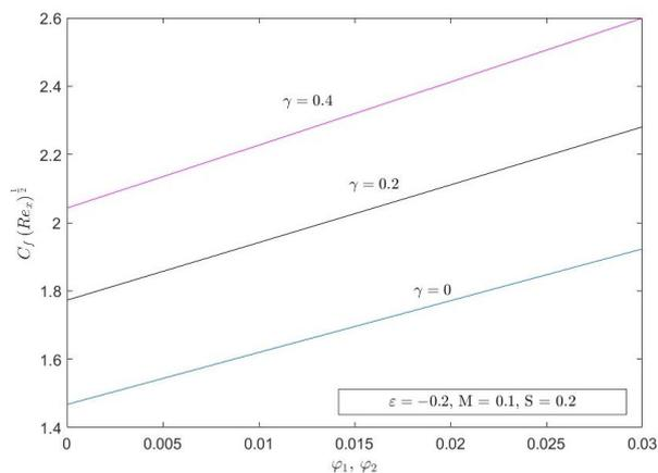
**Fig. 12.** Effect of curvature parameter,  $\gamma$  on local skin friction  $C_f(Re_x)^{\frac{1}{2}}$
