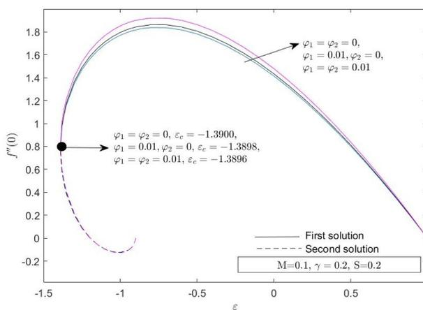
**Fig. 2.** Effect of the volume fraction of nanoparticle,  $\varphi$  on reduced skin friction  $f''(0)$
