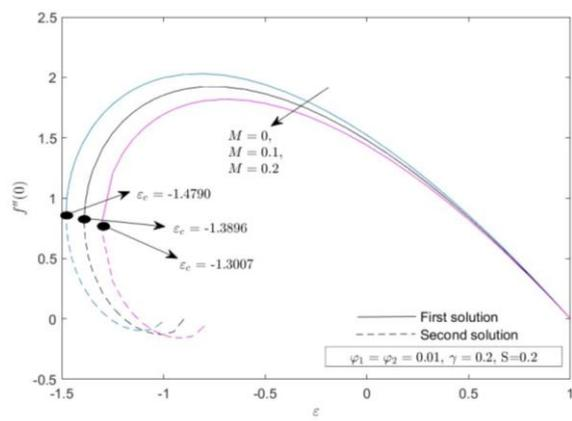
**Fig. 6.** Effect of magnetic parameter,  $M$  on reduced skin friction  $f''(0)$
