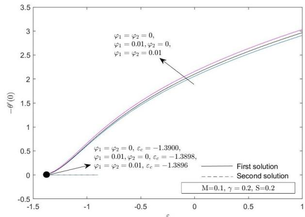
**Fig. 3.** Effect of the volume fraction of nanoparticle,  $\varphi$  on reduced heat transfer  $-\theta'(0)$
