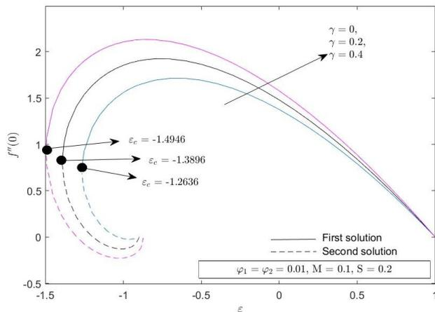
**Fig. 4.** Effect of curvature parameter,  $\gamma$  on reduced skin friction  $f''(0)$
