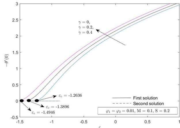
**Fig. 5.** Effect of curvature parameter,  $\gamma$  on reduced heat transfer  $-\theta'(0)$
