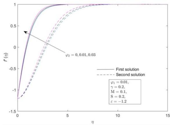
**Fig. 16.** Effect of nanoparticles,  $\varphi_2$  on velocity profile,  $f'(\eta)$
