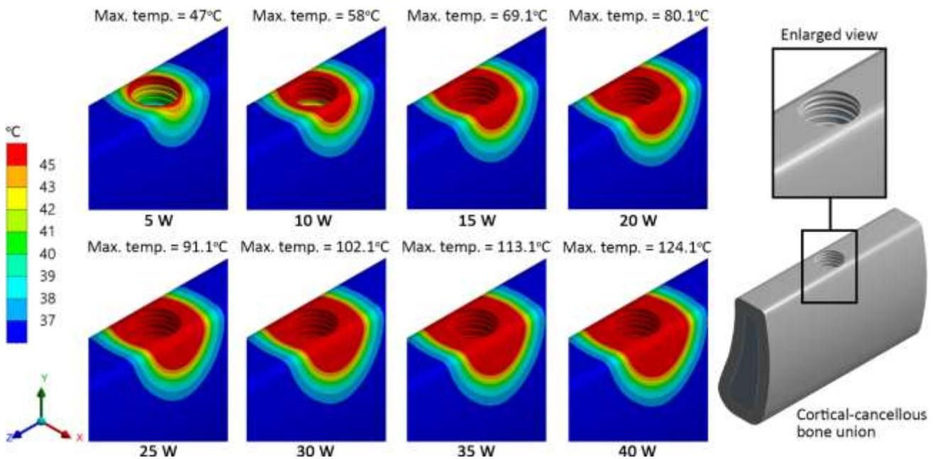
**Fig. 4.** The colour contour plot of temperature levels within the bone in 4 s across all power levels
