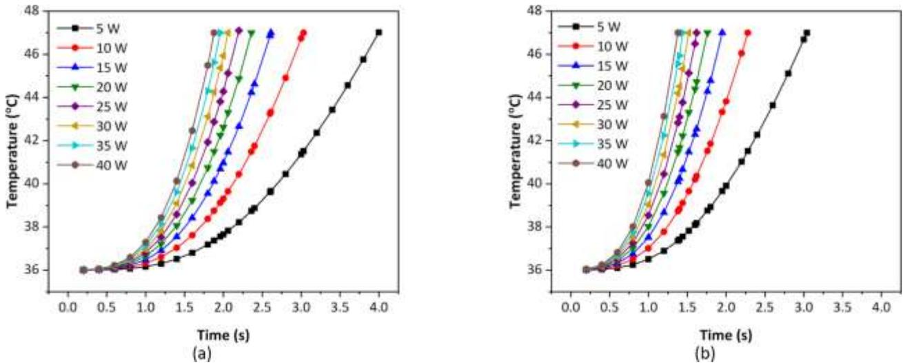
**Fig. 3.** The plot of duration for the (a) cortical-cancellous bone union and (b) implant body to reach 47°C in all power levels
