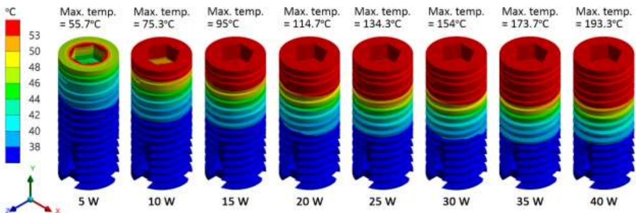
**Fig. 5.** The colour contour plot of temperature levels within the implant body in 4 s across all power levels
