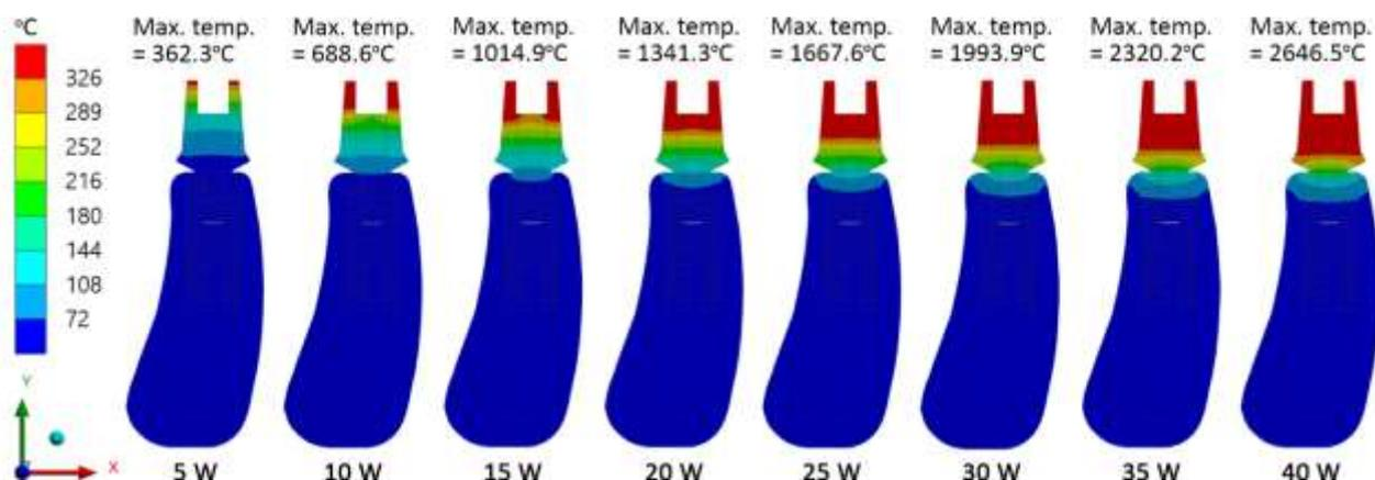
Fig. 6. The colour contour plot of temperature levels within the implant-bone assembly in cross-sectional view in 4s across all power levels
