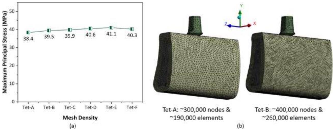
**Fig. 2.** (a) The maximum principal stress plot for all the models. (b) The configuration of tetrahedral meshes for the coarser (left) and more refined (right) models
