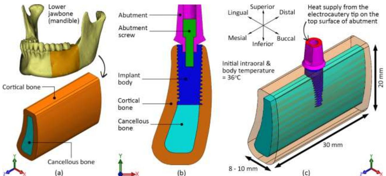
**Fig. 1.** The mandibular bone model consisting of the cortical and cancellous layers. (b) The placement of the implant assembly in the bone. (c) The application of heat at the top surface of the abutment
