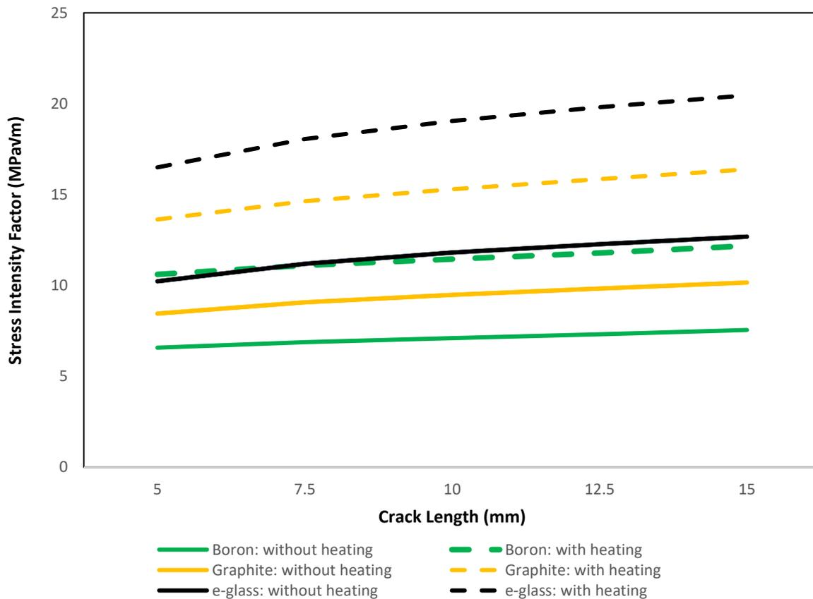
**Fig. 9.** SIF vs thermal heating for different patches
