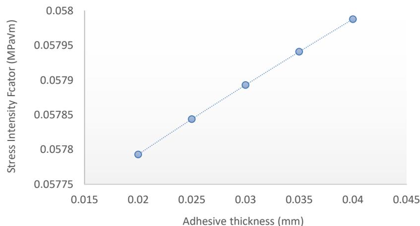
**Fig. 6.** Effect of Adhesive thickness on SIF
