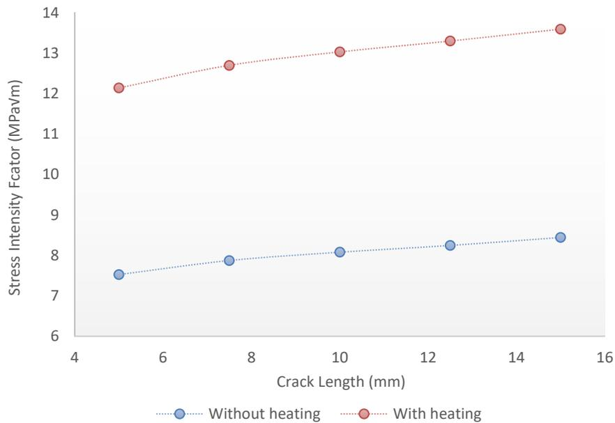
**Fig. 8.** Effect of Thermal heating on SIF
