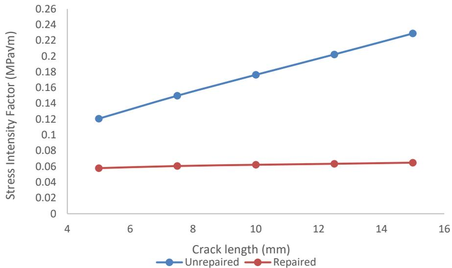
**Fig. 5.** Effect of composite patch and crack length on SIF
