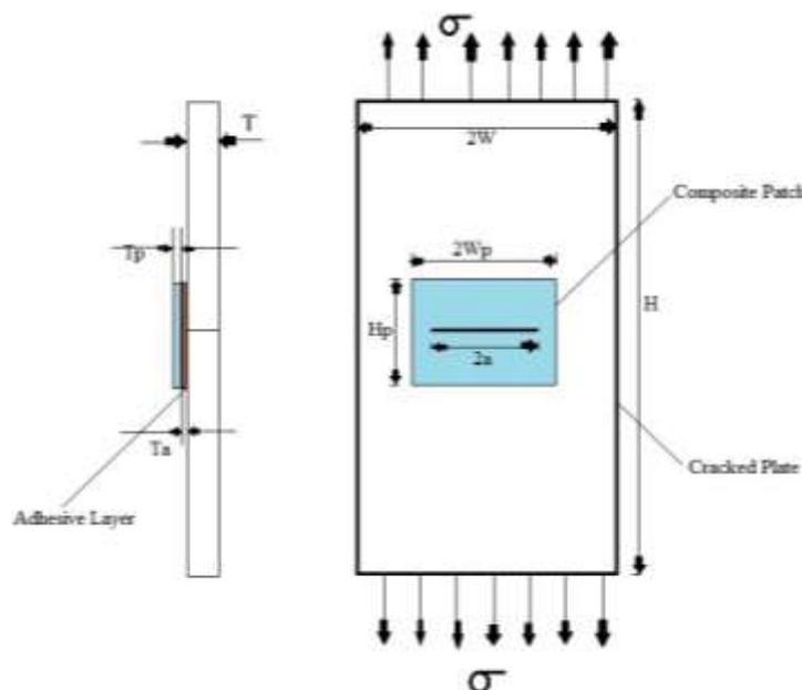
**Fig. 1.** A composite patch bonded by adhesive on a center-cracked plate
