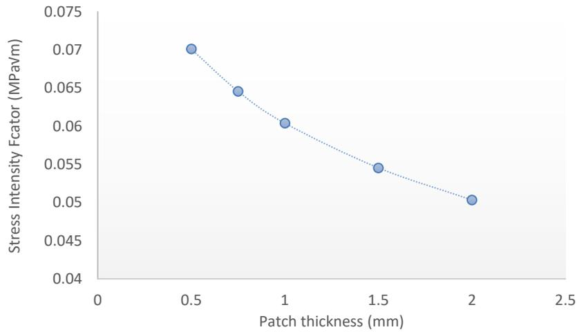
**Fig. 7.** Effect of Patch thickness on SIF
