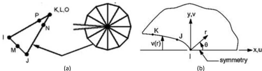
**Fig. 2.** (a) singular element near fracture point and (b) nodes used to calculate the displacements of the fracture tips roughly
