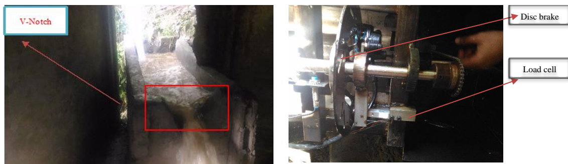
(a) Standard 90-degree V-notch (b) Disc brake dynamometer Fig. 1. The Method of both flow rate (a) and torque (b) measurements
