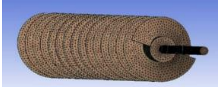
Fig. 3. Meshed model of turbine geometry
