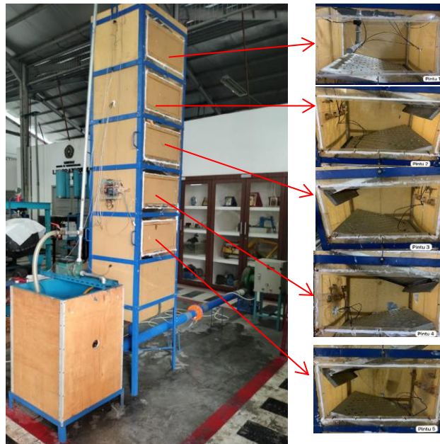
Fig. 4. The image capturing the test cooling tower
